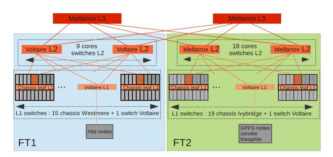
Inside each fat tree, communication between entities are non-blocking. Between the 2 fat-tree, communications are blocking. The link between Level 3 switches has been designed to satisfy GPFS traffic but not to support computation between the two blocks.
